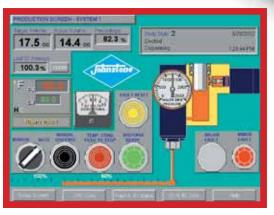
This graphic representation of the dispensing head helps users better understand the system. The AutoStream PC is designed to make viewing system operation and troubleshooting as simple as possible.
