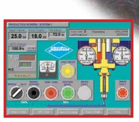
No mixing tube? Nozzle not installed correctly? With the AutoStream PC's graphical interface, you can see these things and many more before they become a problem.
